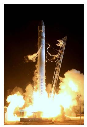
system, dubbed "Niagara," is activated. Its purpose is to suppress acoustic waves that radiate from the engine plumes, thereby mitigating the effect of vibration on the rocket. Fifty-three water nozzles set low on the launch pad provide a curtain of water flowing at 113,500 liters (30,000 gallons) a minute. The system is deactivated within 20 seconds of T-0.
