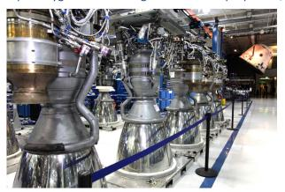
thrust at liftoff, rising to 716 kilonewtons (161,000 pounds) as it climbs out of Earth's atmosphere. Merlin's thrust-to-weight ratio exceeds 150, making the Merlin the most efficient booster engine ever built, while still maintaining the structural and thermal safety margins needed to carry astronauts.
