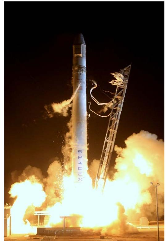
Three seconds before launch, the nine Merlin engines of the first stage ignite. The rocket computer commands the launch mount to release the vehicle for flight, and at T-0:00 Falcon 9 lifts off, putting out 850,000 pounds of thrust.
