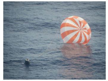
SpaceX will use a 150-foot boat equipped with an A-frame crane and two inflatable boats to perform recovery operations. On board will be approximately a dozen SpaceX engineers and technicians as well as a four-person dive team. Once Dragon splashes down, the team will first secure the vehicle and then place it on deck for the journey back to shore.
