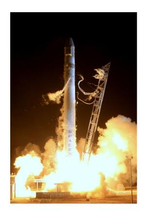
system, dubbed "Niagara," is activated. Its purpose is to suppress acoustic waves that radiate from the engine plumes, thereby mitigating the effect of vibration on the rocket. Fifty-three water nozzles set low on the launch pad provide a curtain of water flowing at 113,500 liters (30,000 gallons) a minute.
