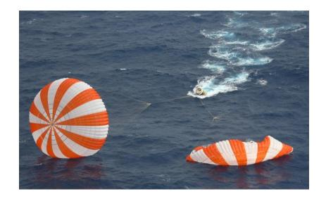
spacecraft's descent to approximately 4.8 to 5.4 meters per second (16 to 18 feet). Even if Dragon were to lose one of its main parachutes, the two remaining chutes would still permit a safe landing.
