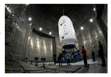
There are two halves to the fairing. One side is passive, and one is active with all actively controlled systems.
