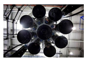
The new layout also provides individual protection for each engine, and further protects other engines in case of an engine failure. It significantly reduces both the length and weight of the Falcon 9 first stage. With this design, Falcon 9 is also prepared for reusability – the Octaweb will be able to survive the first stage's return to Earth post-launch.
