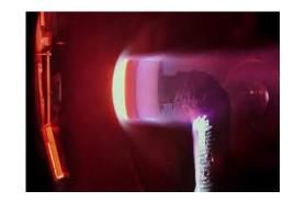
A sample if PICA-X being tested at NASA's Arc-Jet Facility [13]
