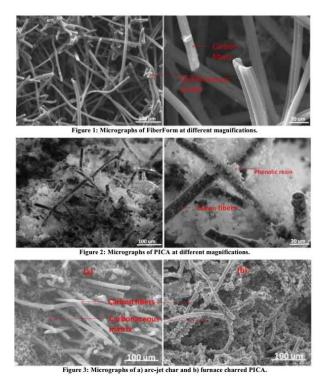
Various magnifications of PICA during a heat test [25]
