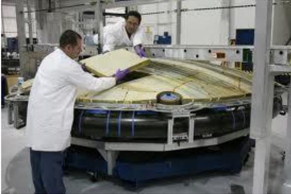
Tiled PICA-X being applied to the Dragon's heat-shield carrier [13]
